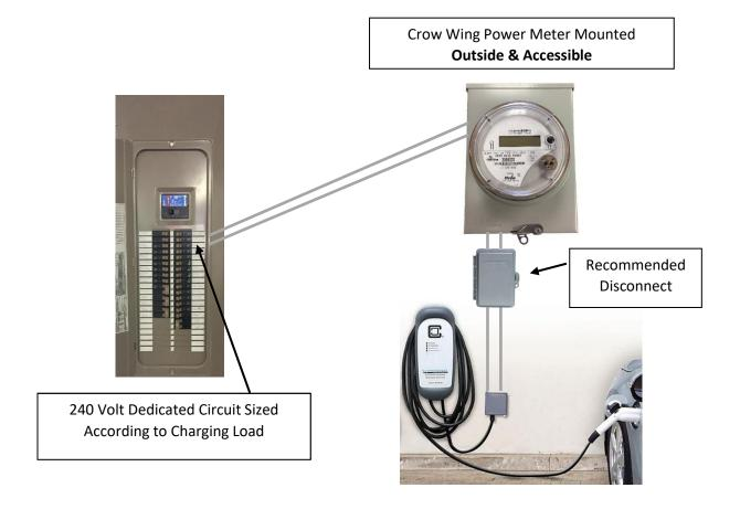
Note: ALL EQUIPMENT must be installed and inspected meeting the requirements of the National Electric Code. Meter bases for Level 2 chargers may require a local breaker style disconnect.
